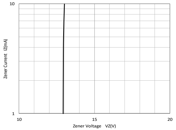
Fig 2: Zener Breakdown Characteristics
