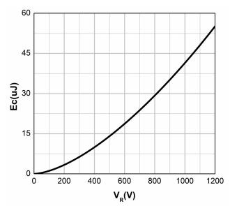
Figure 5. Capacitance Stored Energy
