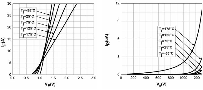
Figure 1. Forward Characteristics
