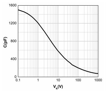
Figure 3. Capacitance vs. Reverse Voltage
