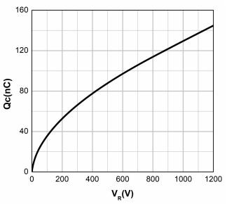
Figure 4. Total Capacitance Charge vs. Reverse Voltage
