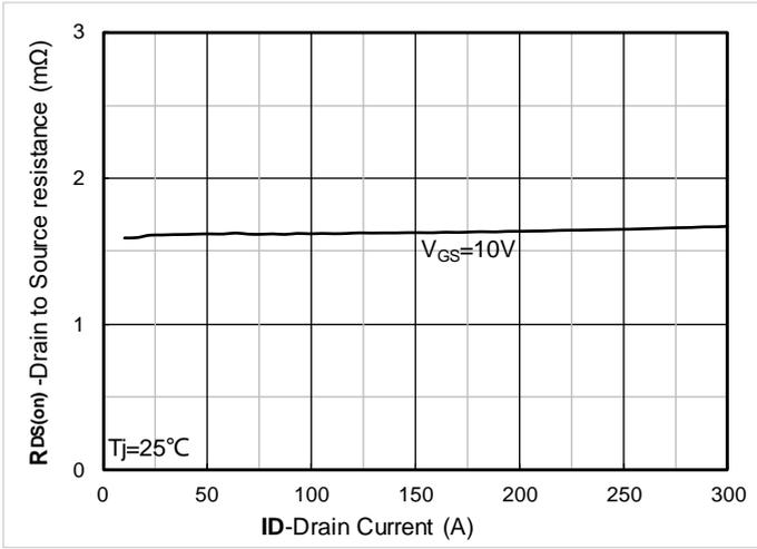
Figure 7. RDS(on) vs. Drain Current; typical values
