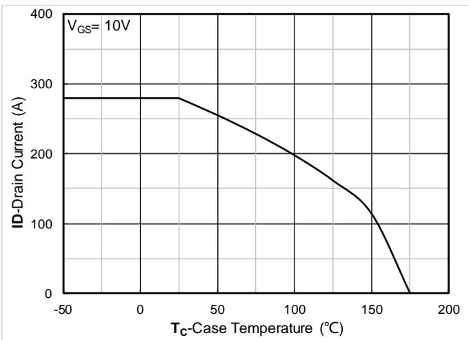
Figure 11. Current dissipation
