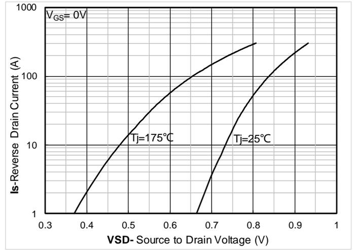
Figure 8. Forward characteristics of reverse diode; typical values
