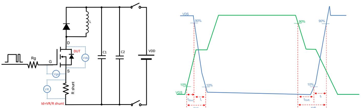
Figure C. Resistive Switching Test Circuit & Waveform
