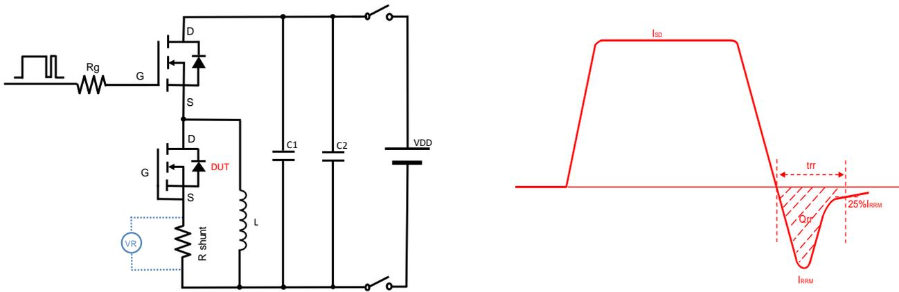
Figure D. Diode Recovery Test Circuit & Waveform
