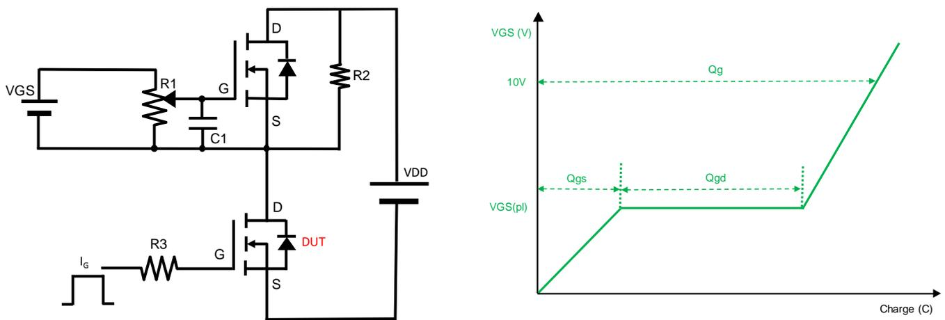
Figure B. Gate Charge Test Circuit & Waveform
