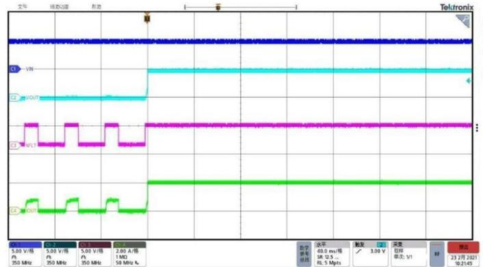
output short circuit recovery with 2.5Ω load
