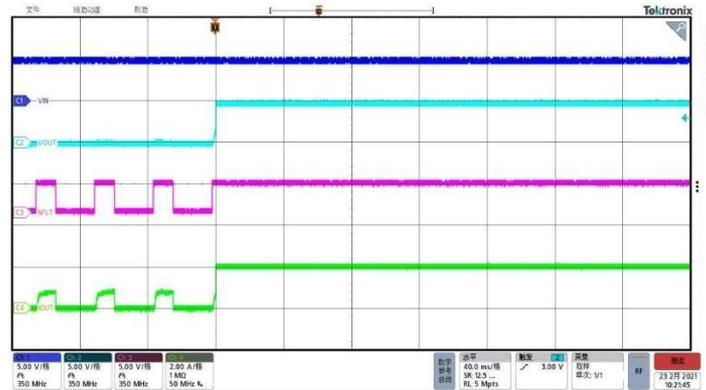
output short circuit recovery with 2.5Ω load
