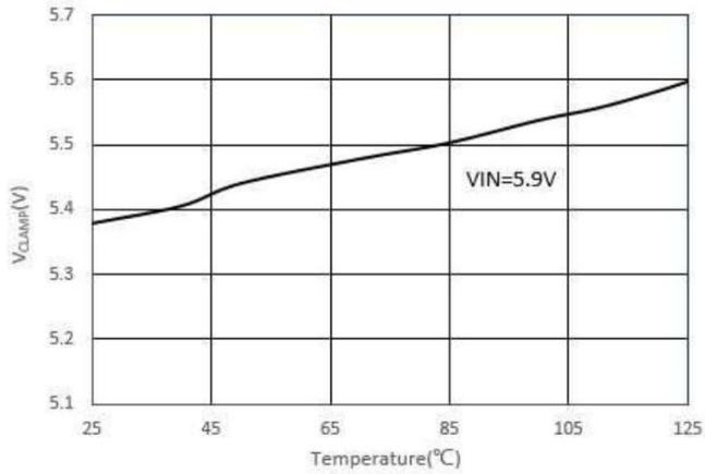
**V<sub>CLAMP</sub> vs. Temperature**
